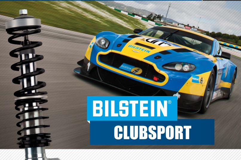
Derived from years of motorsports experience, the BILSTEIN Clubsport® is our most advanced coilover kit. Featuring a 2-way damping system, the BILSTEIN Clubsport® allows 10 rebound and 10 compression settings to be adjusted independently, accurately, and quickly via easily accessible adjusters.
