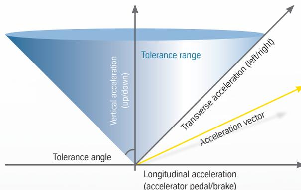
When set to **Auto** mode, the three-axis acceleration sensor reads the vehicle acceleration, cornering and vertical forces, and adjusts suspension damping in real time. This app includes a graphic display that illustrates longitudinal and lateral acceleration along with the ability to precisely adjust acceleration thresholds, switching times and filter parameters when creating custom settings.
