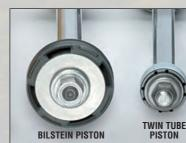
Monotube VS. Twin Tube Shock Design The photo on the left dramatically illustrates the size difference between the working piston inside a Bilstein monotube shock and one found in a typical "twin tube" shock.
