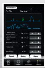
The customer can adjust the sensitivity to vertical acceleration (up-and-down movement), horizontal acceleration (transverse acceleration to the left and right) and longitudinal acceleration (accelerating and braking) through their iRC application.
